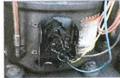
Figure 3-17: Loose connection causes arcing and short-cut
