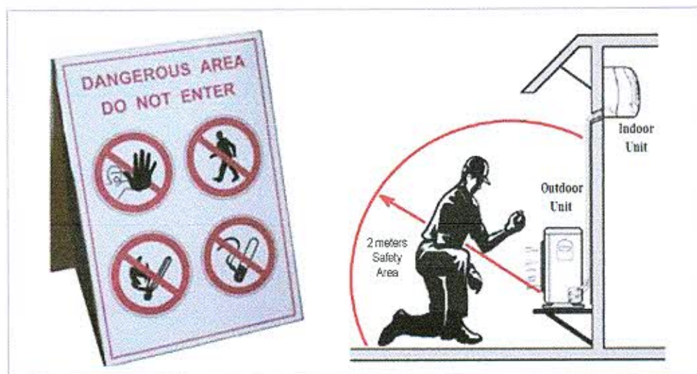
Figure 3-1: Designated work area where potential Sources of Ignition (SOI) must not be present during service works
