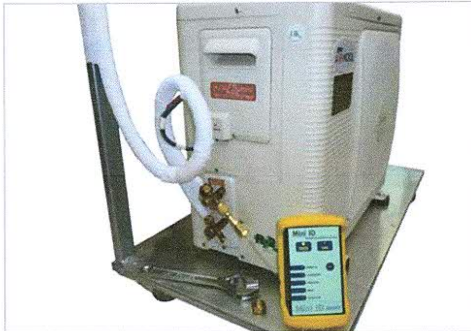
Figure 3-2: Example testing the "old" existing HCFC R22 refrigerant quality
