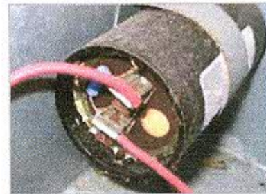
Figure 3-18: Not acceptable capacitor may cause short-cut and
